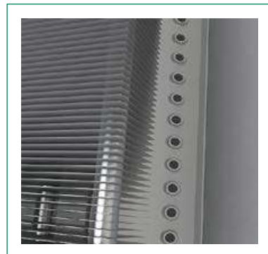
Figura 6: Boquillas de aire de alta eficiencia Figure 6: High Efficiency Air Nozzles
